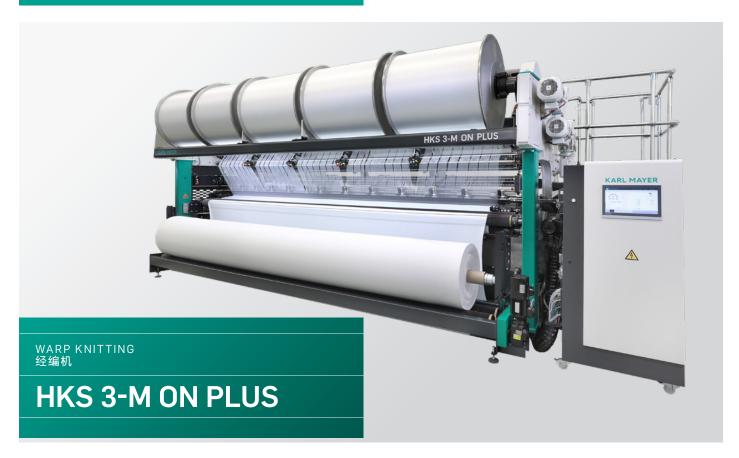
High-performance tricot machine with highest possible variety in mesh density and layers with "PLUS Equipment". Extended sinker movement for high flexibility in patterns. 配备PLUS Equipment的高性能特里科经编机, 拥有更广泛的线圈密度可调范围, 优化的沉降摆臂调节区间, 更佳的产品灵活性
